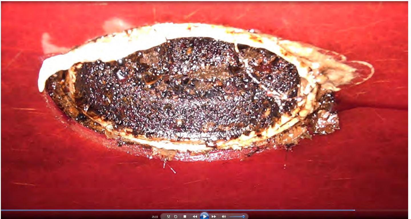
Figure 4-4: Corrosion in bung (21:11)
