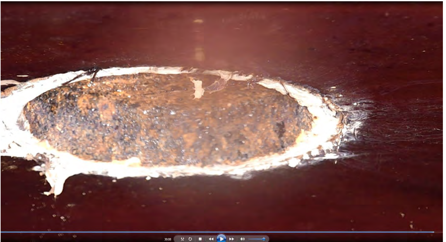
Figure 1-12: Corrosion in bung (30:08)
